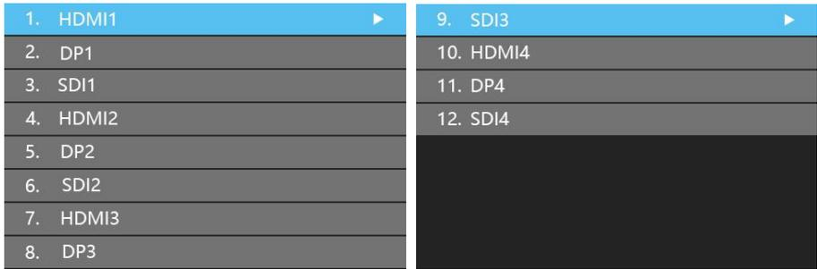
Enter the clip interface of “HDMI1/2/3/4” or “DP1/2/3/4” or “SDI1/2/3/4” , press the knob/OK to turn on/off cropping. Set X, Y, width, and height of the input signal by knob then save the data.
