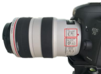
Fig.4-4 Adjust the focus mode
