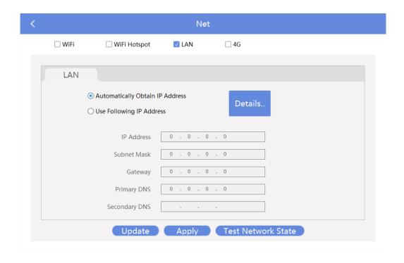
Take LAN as an example, the player will automatically obtain the IP address after connecting to the Ethernet cable.
